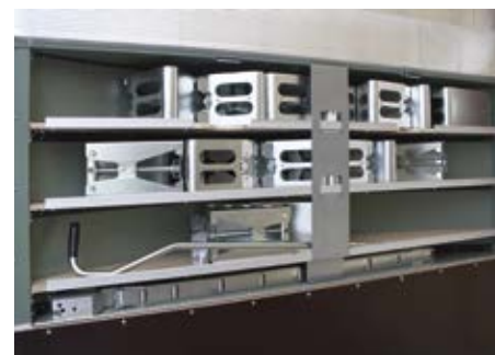
Storage cases – built into the bulkhead in this case – make sure that the necessary parts are available at any time.
