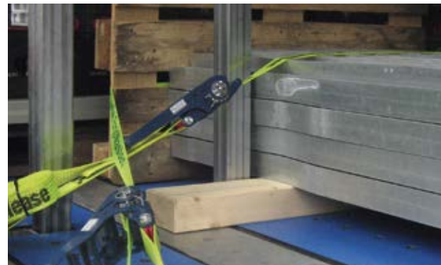
Positive locking on the side and at the front, with the load lashed down.
