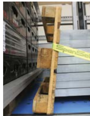
A supporting pallet held in place by belts is a simple solution for securing loads with positive locking.
