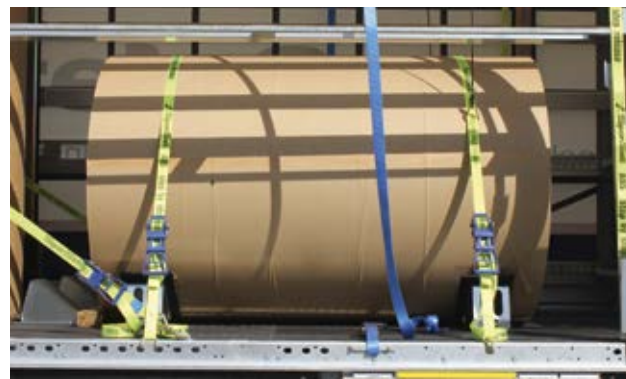
Horizontal paper rolls positioned perpendicular to the driving direction. Lashed down with two straps and secured at the front with securing chocks.
