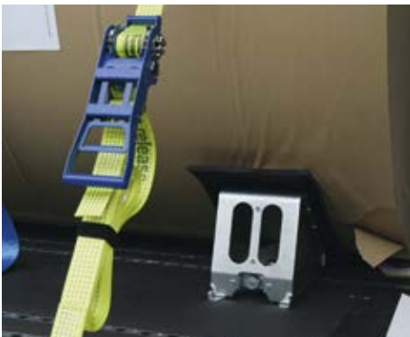
Chocks lock rolls of paper, while lashing belts increase the contact pressure.
