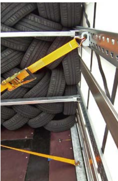
The necessary diagonal restraints are anchored in the side steel slats using perforated grids and the lashing points in the trailer frame.
