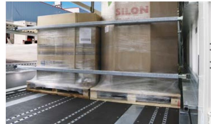
Horizontally used support slats provide the side interlocks for palletised octabins. Clamping beams secure the load longitudinally.
