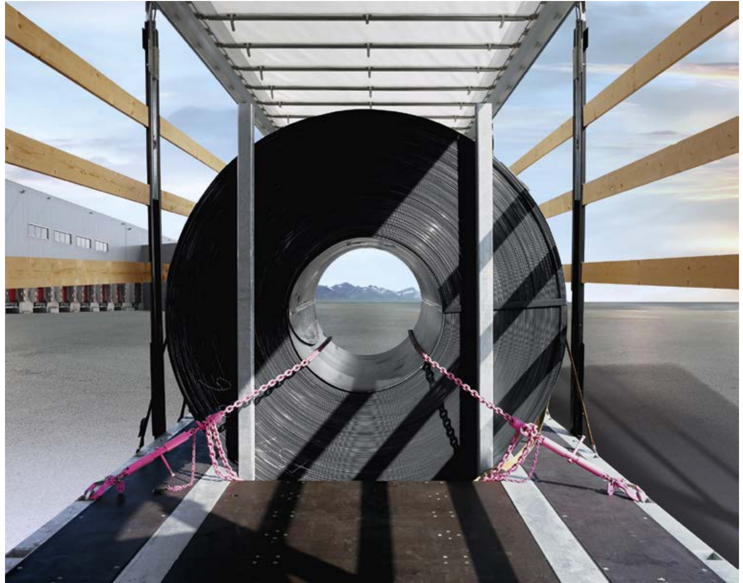
Positive locking of a steel coil using special recess, inserted stanchions and chains anchored in heavy-duty lashing eyes.
