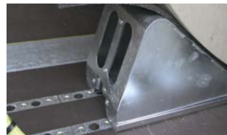
Positive locking blockade of the roll using special chocks, in combination with anti-slip mats.
