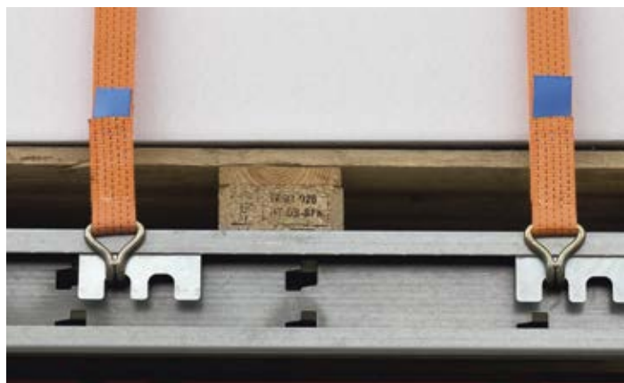
Lashing straps can be firmly secured to the I-beams on the second level.
