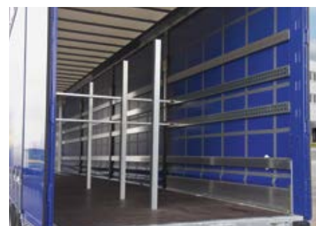
For transporting profiles and bar materials additional stanchions and steel support slats with horizontal beams are included.
