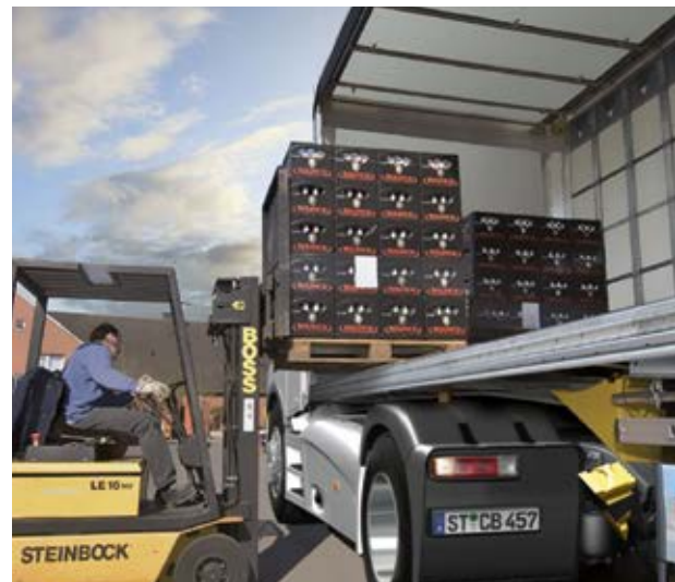
Beverage cases with positive locking can be safely transported without lashing down when using the appropriate equipment.
