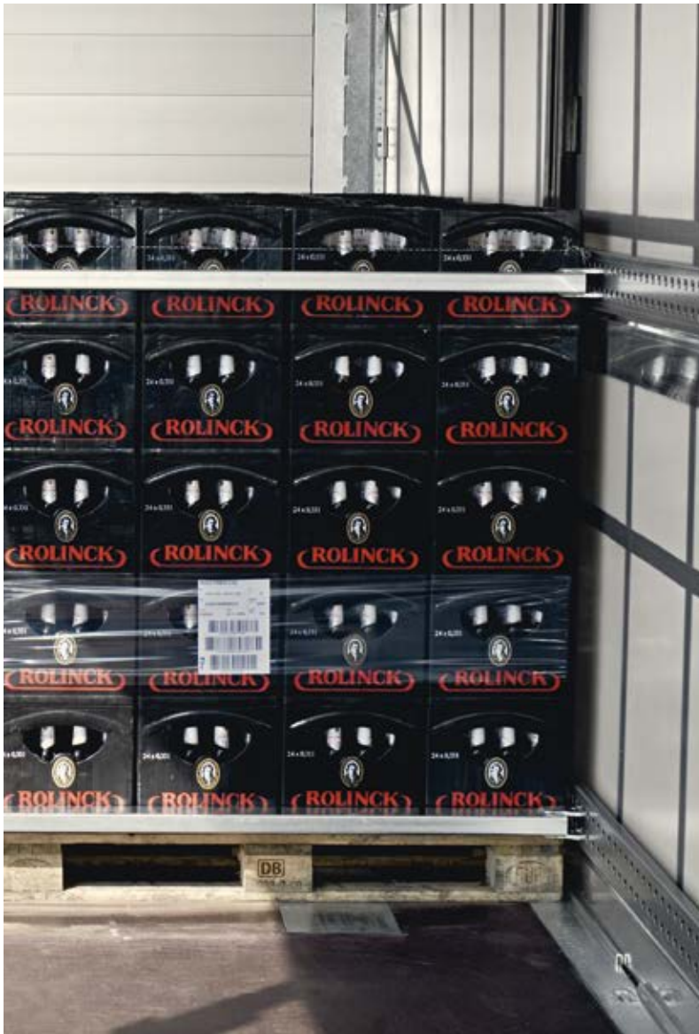
Transverse beams at the front and rear of the freight secure partial loads against sliding longitudinally.
