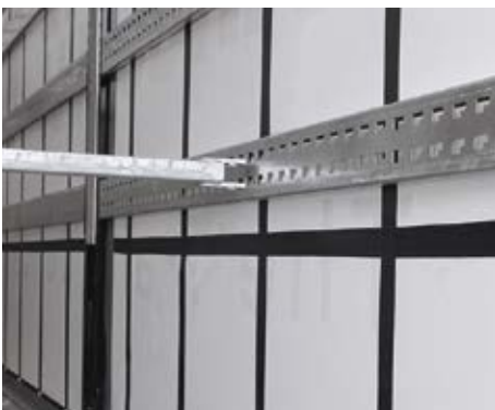
Tarpaulin with diagonal reinforcing straps and load securing beams for partial loads.
