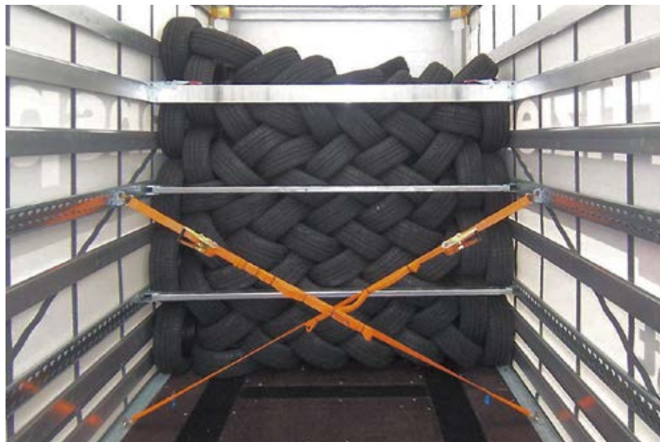
Loose tyres in a laced arrangement tend to settle during transport and exert strong sideways pressure. The structural stability of the sides must be ensured.
