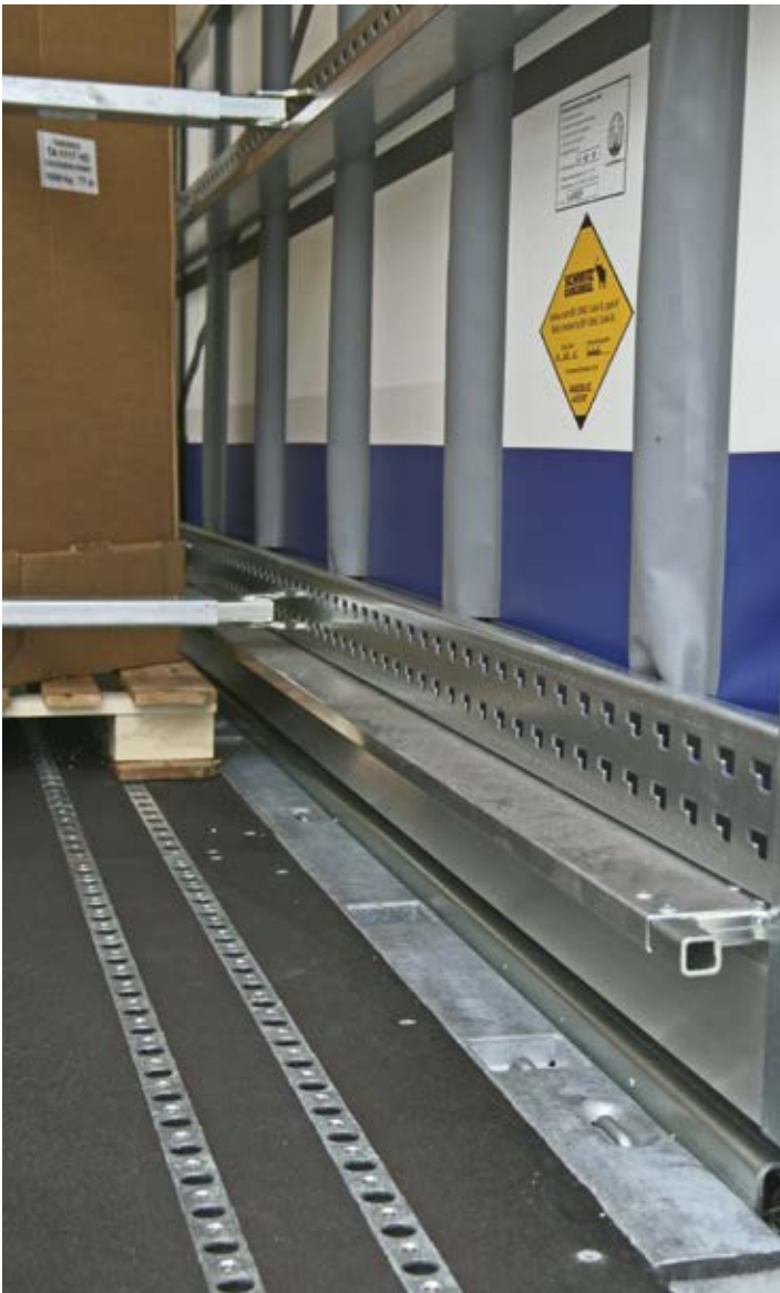
Gaps to the side of the load can be filled quickly and safely using folding laths.
