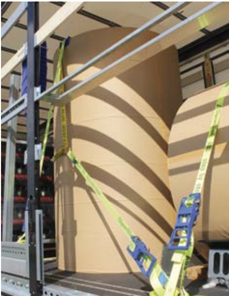
Upright paper rolls, secured through direct lashing with the head strap and lashing down.
