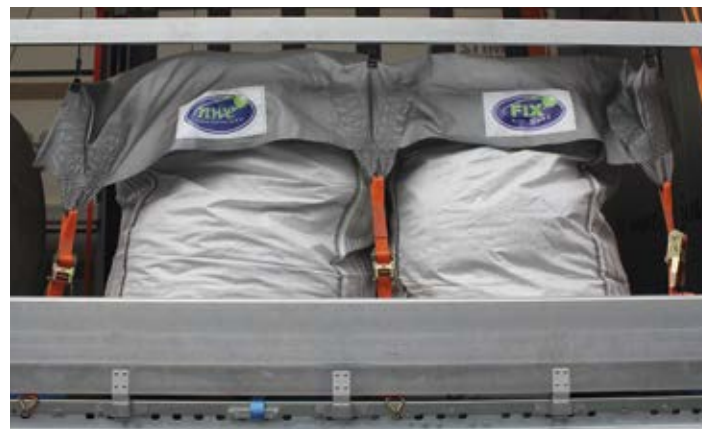
Positive locking for pliable big bags: Our aluminium and tarpaulin side laths with lashing belts.
