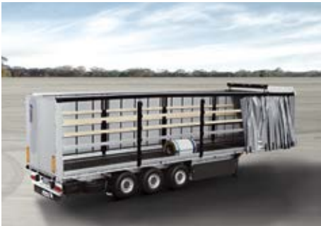
The coil well defines the ideal loading position.
