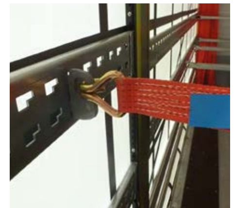
Using suitable adapters, belts can be hooked into the side grid in the steel laths.
