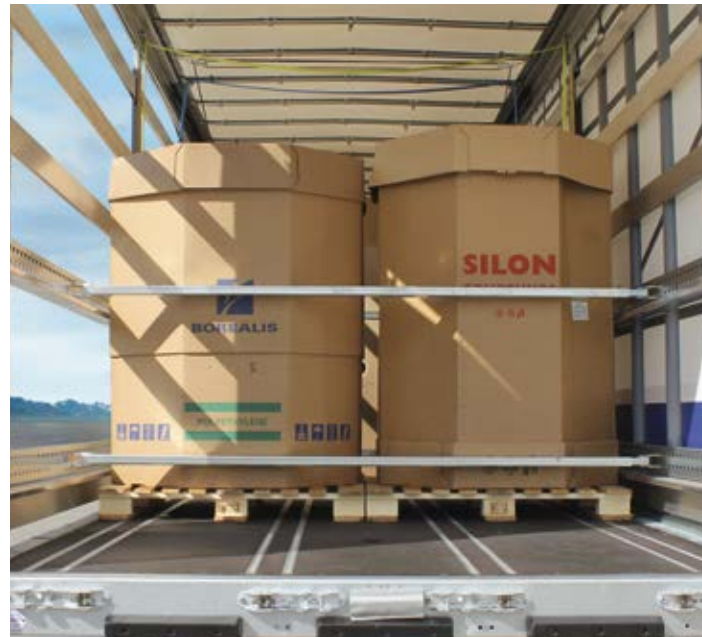
Ideally, octabins on pallets are secured using positive locking and cross beams.
