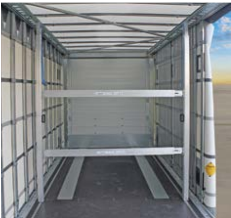
A system of supports and locking bars for free positioning.
