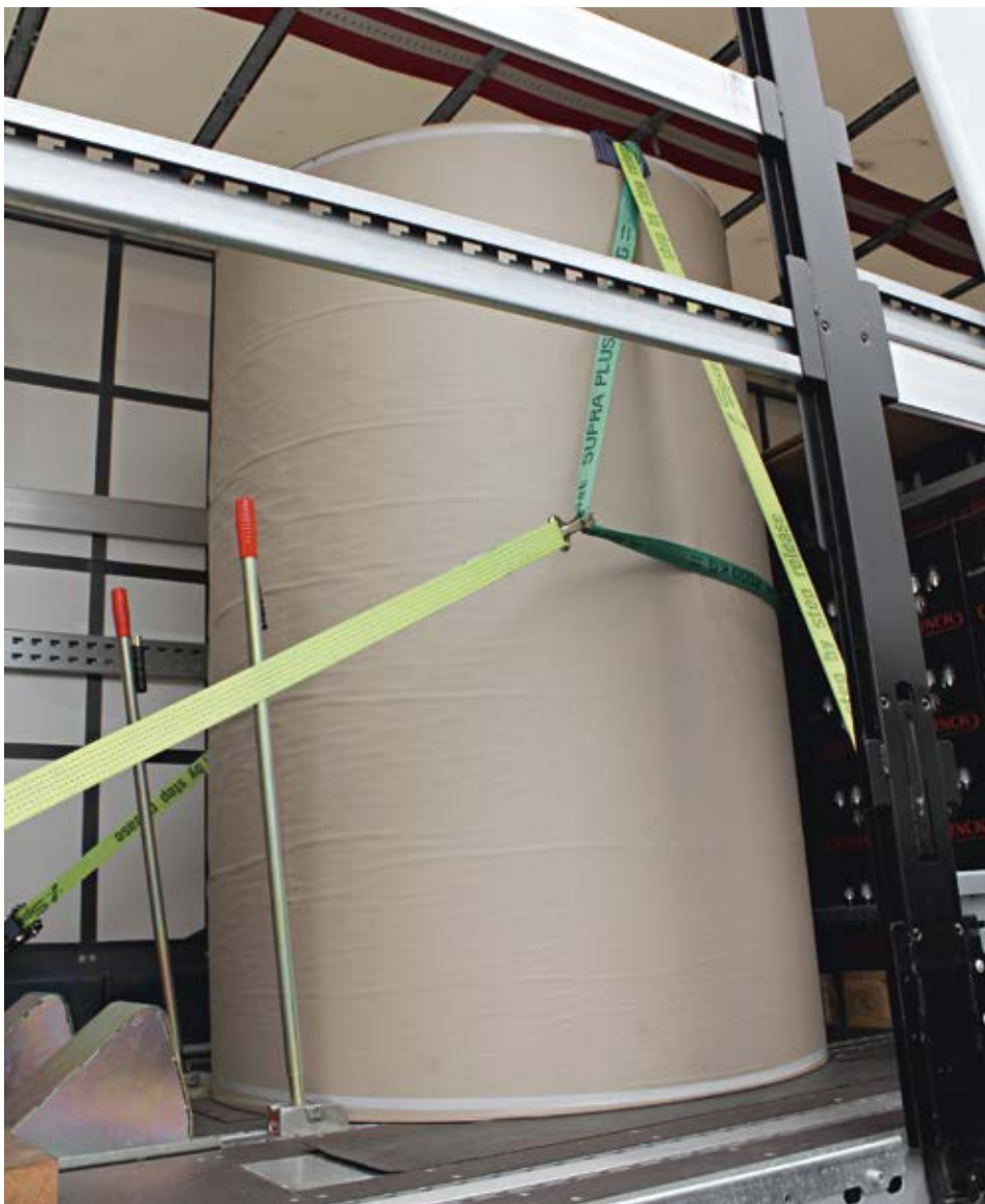
Transportation of paper rolls using positive and forced locking. The head strap of the standing rolls also secures against tipping.
