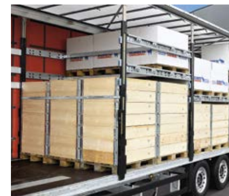
Cross beams can be mounted on the stanchions and in the double-decker side support beams for positive locking of partial loads.
