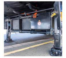
Battery Power Pack with a capacity of 32kW/h. The lithium iron phosphate battery transformer has a self-sufficient running time of approx. 4.5h and requires approx. 2h for a full charge.
