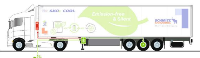
Charging options for the battery in the support winch of the S.KOe semitrailer box: - stationary via the CEE socket on the underside of the refrigeration unit S.CUe - on the move generatively or recuperatively (when braking) through the e-axle in the ROTOS chassis.
