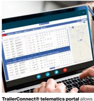
refrigeration unit control with setpoints for operation, temperature and alarm management. It provides information about the battery's state of charge, the vehicle's position and is used for route planning.
