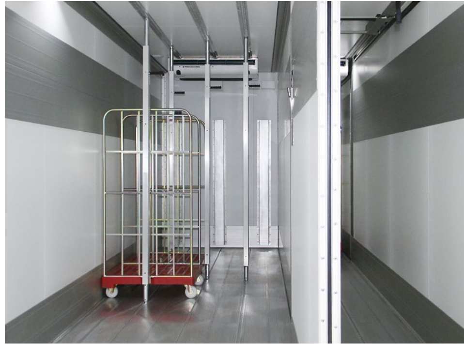
Vertical telescopic beams with special feet for load securing on the multifunctional floor.
