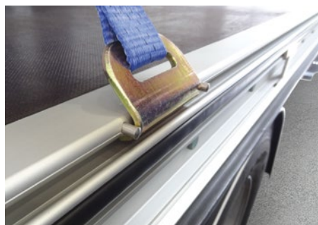
Practical clamping rails for freely positionable, self-clamping load securing belts at the top and the bottom on the out of frame.
