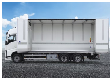
Side loading and unloading along the full length or from the rear using the tail lift.
