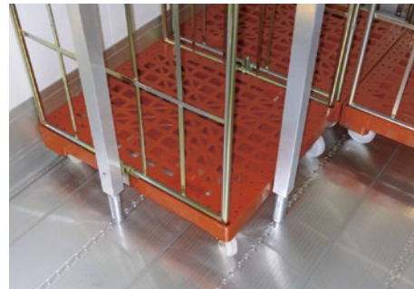
The flush-mounted locks of airline rails in the roof and floor simplify load securing with vertical telescopic beams.
