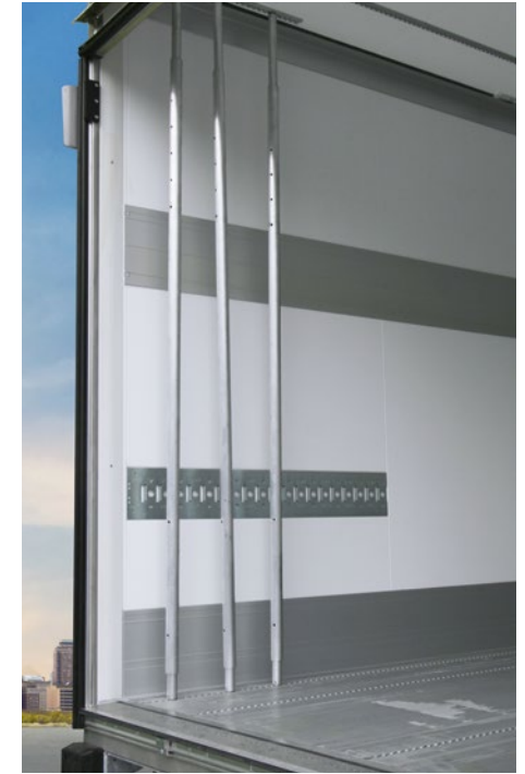
Easily accessible and simply secured until needed – side locking bars.
