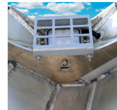
Interior lighting of the aluminium volume body enables the cleaning or handling of palletised freight, even with the tarpaulin closed.
