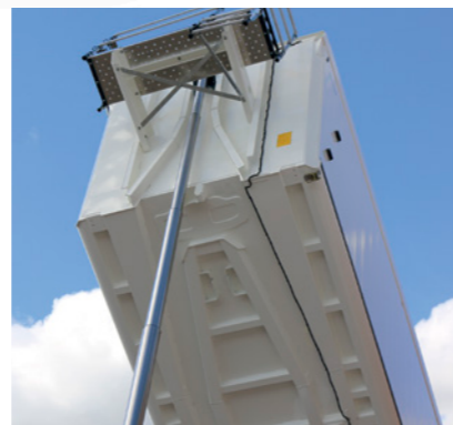
Partially recessed chassis neck area in the body floor assembly for a lower body loading height and a reduced overall height.
