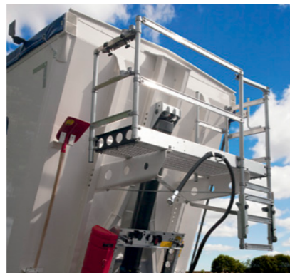
Height-adjustable working platform with anti-slip floor, trough boarding aid and park position for hydraulic hose.
