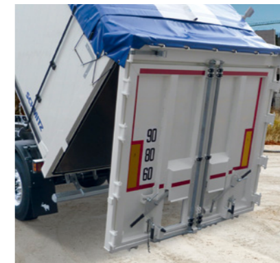
Emptying with the tarpaulin closed using the pendulum function of the combi-door saves time when unloading.
