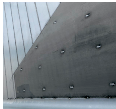
Additional wear plates in the rear increase the service life of the body.
