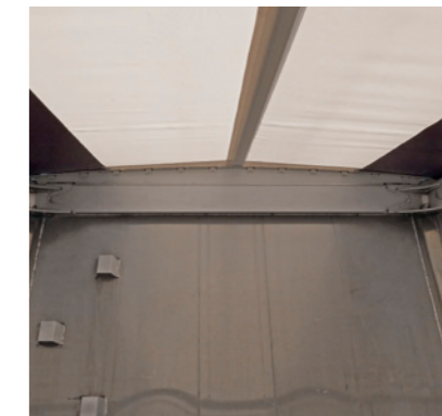
The arc-shaped design of the roller tarpaulin with a stabilising central tube prevents water from collecting.
