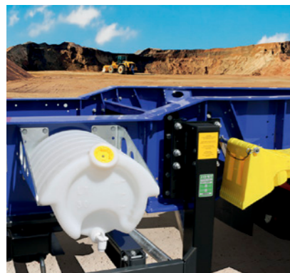
The offset in the neck area of the chassis (step-frame) allows for a reduced loading height.
