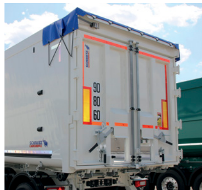
Combi-door with a pendulum frame, two door wings and two grain sliders.
